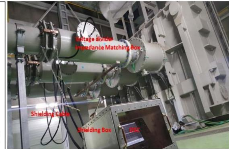
Figure 2 : VFTO measurement arrangement using CVD sensors in 765 kV GIS
