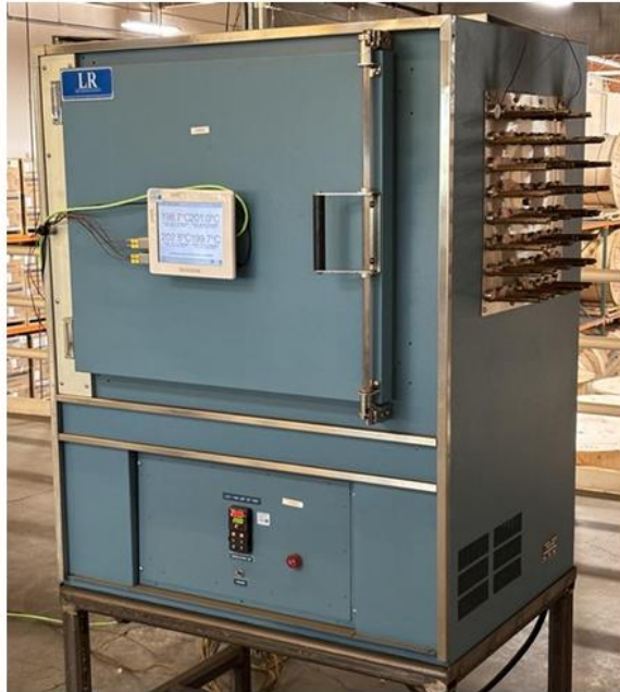
Figure 2. Representative air circulating oven used for temperature exposures.
