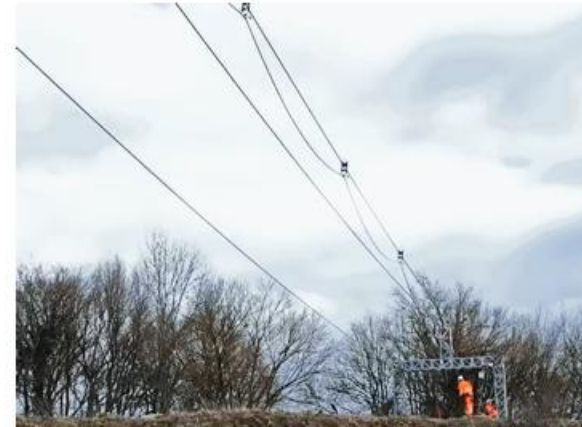
Figure 8 – Field Test “conductor break” for single conductor (left) and bundled conductor (right)
