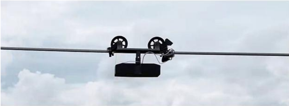
Figure 1 - Robotic application for in-situ SSC deployment.
