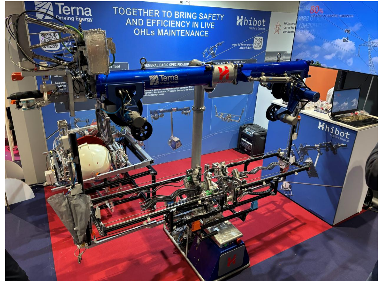
Picture: Hibot inspection robot for Terna (TSO Italy)
