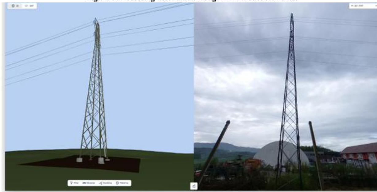
Figure 8: Comparison of 360° photo and BIM model in CDE.
