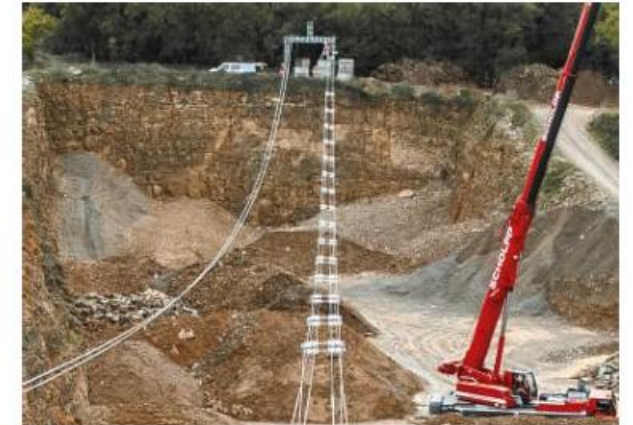
Figure 8 – Field Test “conductor break” for single conductor (left) and bundled conductor (right)
