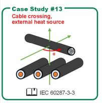
Cables of 2 circuits with crossing heat source (under a given angle).
