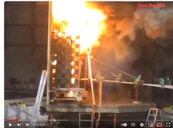
Viewsafe™ - Internal Arc Classification Test - 50kA for 1 second @ 11kV
