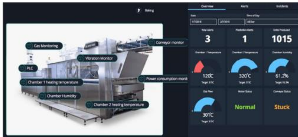
Figure 4: BIM integration with Internet of Things (IoT) for asset monitoring and predictive analytics.
