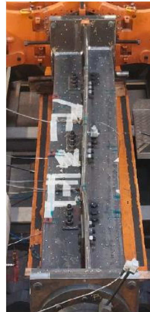
Deformed S460 steel member
