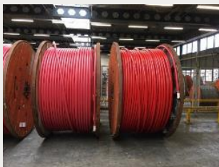
rPE sheathing grades for MV cable
