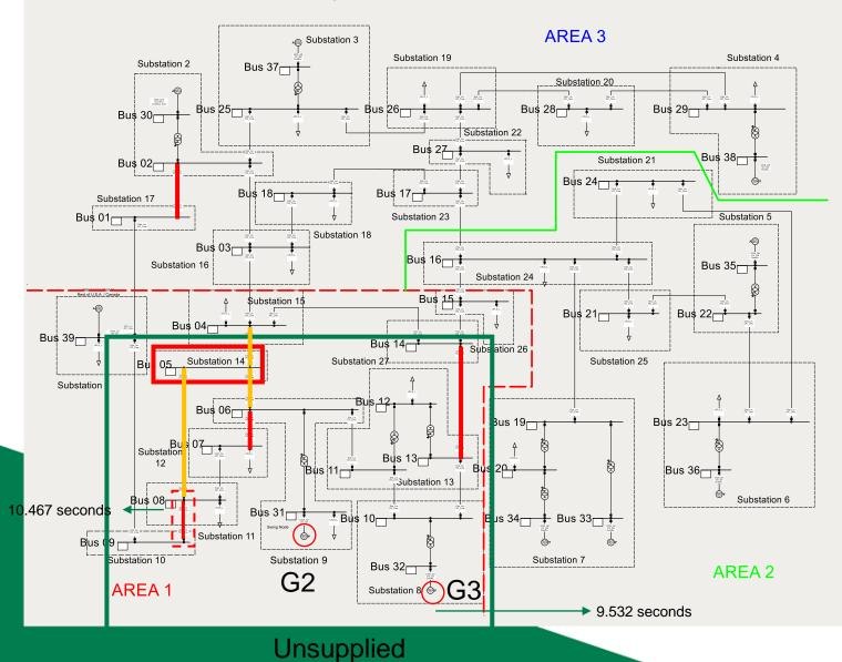
Generators G2 and G3 trip due to ROCOF protection
