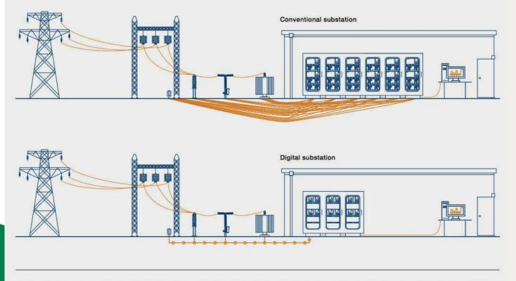
\*The digital process bus is managed by the IEC 61850-2 subsection of the standard for digital substation communication. It underpins the true digital substation and requires a new approach to substation architecture, design and construction.
