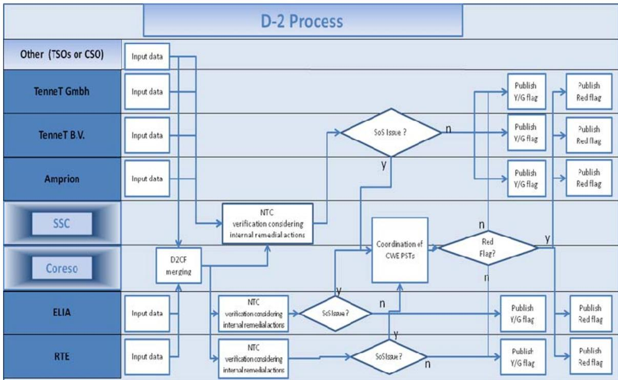
Fig. 3: PST coordination in the D-2 process
