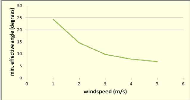
Figure 4 Effective wind angle as a function of wind speed.
