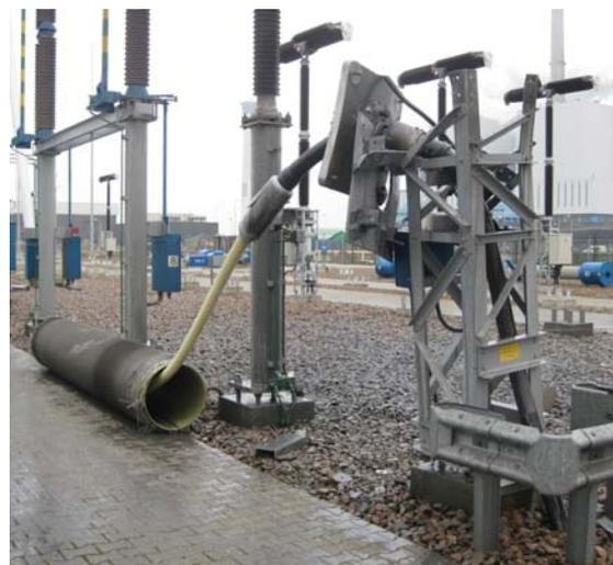
Figure 2: Failed 380 kV cable termination.
