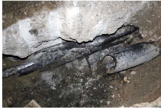
*Figure 5: thermal influence between two phases after a fault at a 110kV cable.*
