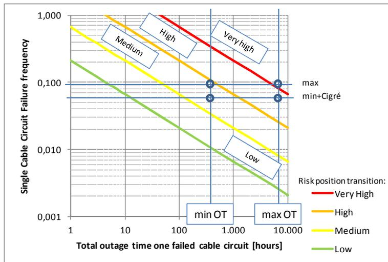
Figure 1: Relation between total outage time to repair one failed cable circuit, the failure frequency of one single cable circuit and the risk position of a TSO if the impact on security of supply is catastrophic.
