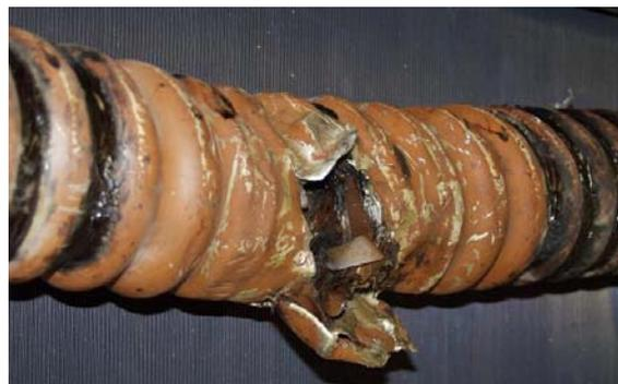
*Figure 6: damage at a 380kV cable from digging work.*
