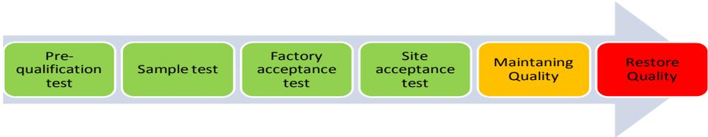
Figure 4: Structure of the quality management system. The green blocks lead to quality built-in the cable system and should be aimed for. The orange block contains actions to maintain quality during operating the cable system. The red block contains methods to restore the quality after a failure.
