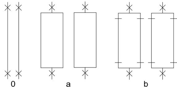
Figure 7: Different configurations for double circuit systems. 0 = double overhead line circuit, a = double cable circuit, b = double cable circuit with the possibility to isolate a failed cable. The "X" represents circuit breakers, the "-" represent disconnecting options.
