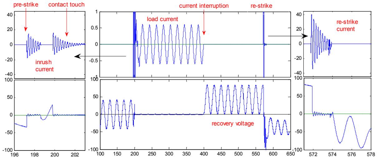
Fig 9: Current (top, [kA] and voltage across the interrupter (bottom, [kV]) during a single phase back-to-back test. Time in ms. Left: Pre-arcing period enlarged, middle: complete sequence, right: re-strike period enlarged.
