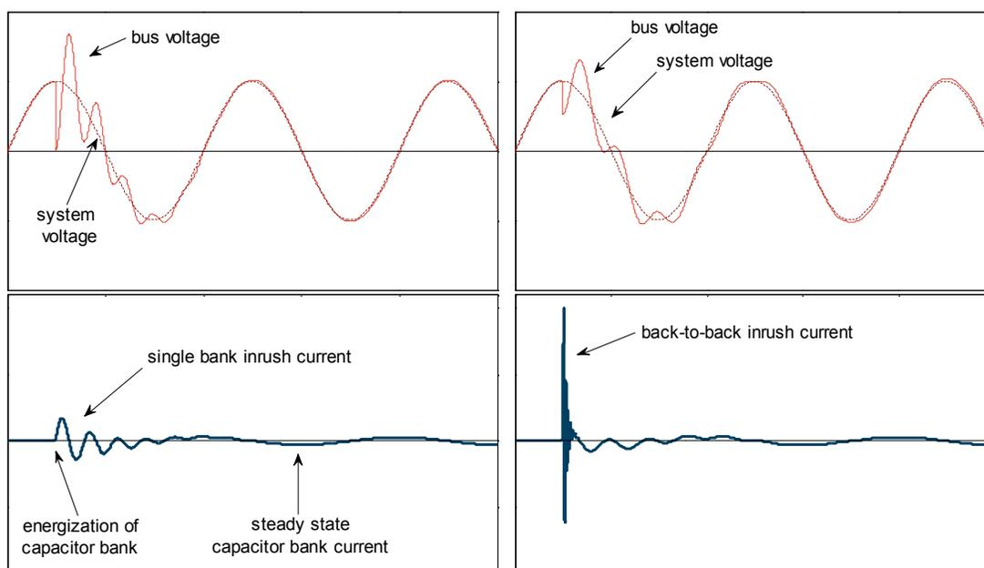
*Fig. 1 Single cap bank energization (left) and back-to-back cap bank energization (right).
