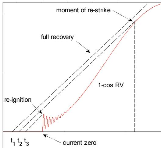
Fig. 2: Re-ignition and re-strike in relation to voltage jump
