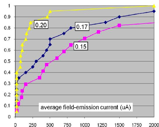
Fig 8: Cumulative "smaller than" plot of FEE current in three interrupters. Indicated figures are fraction of test with re-strikes
