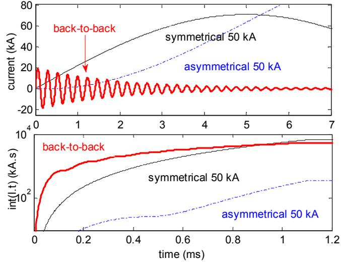
Fig. 6: Currents (top) and integrated current (bottom) during pre-arcing period
