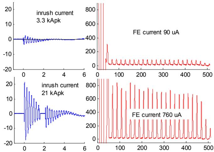
Fig 10: Effect of low (top) and high (bottom) inrush current on FEE current after interruption of 400 A capacitive current
