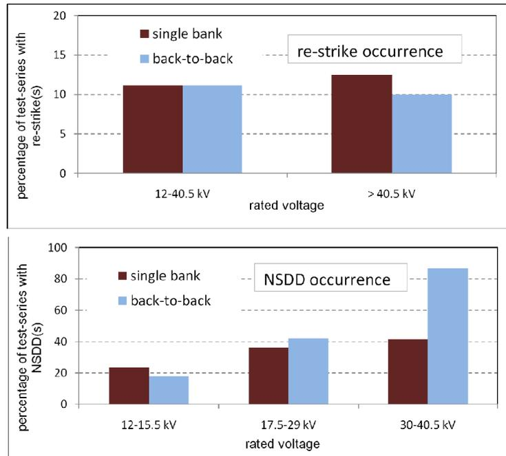
Figure 5: Percentage of test-series in which re-strike (top) and NSDD (bottom) occurred..
