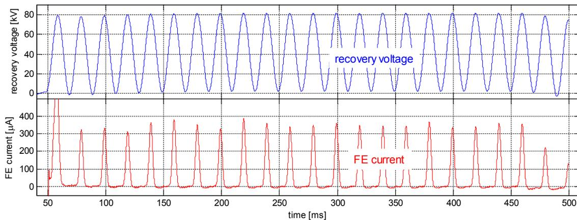
Fig. 7: Field electron emission current (bottom) during recovery voltage (top) of 36 kV vacuum interrupter after interrupting 400 A capacitive current with making at 20 kA back-to-back inrush current
