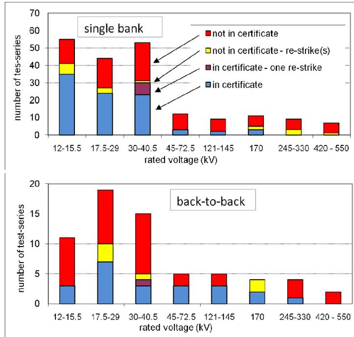
Figure 4: Numbers of cap bank test-series in voltage classes for single bank (top) and back-to-back (bottom) tests.
