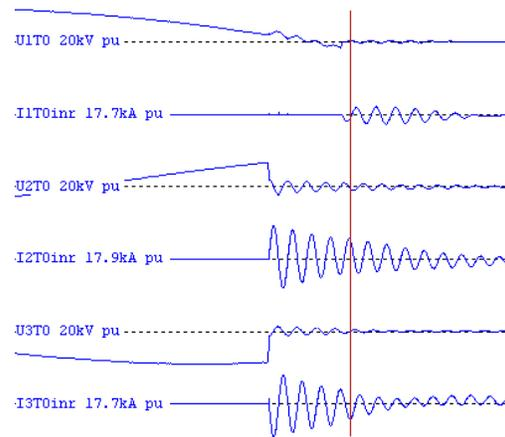
Fig. 3: Three-phase inrush current in lower two phases only
