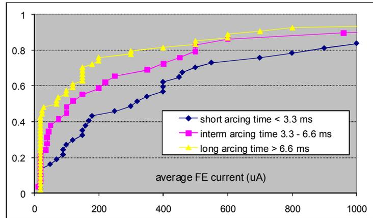
Fig. 11: Cumulative "smaller than" plot of FEE current for three classes of arcing time.
